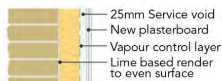
Internally insulated stone wall
