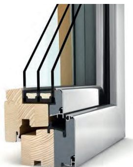
Triple glazed opening sash – timber frame with aluminium cladding and two seals (Source: Internorm)
